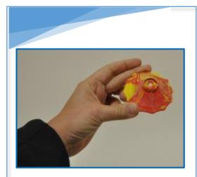
Hold the Dropper Popper with the "bulge" pointing upward. Its stored energy will be released when you drop it, causing the popper to bounce up beyond the height at which it was dropped.
